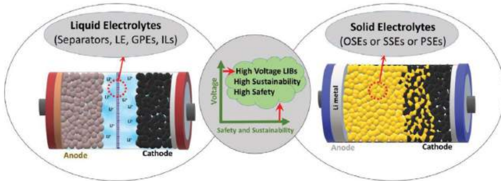
Figure 1. Schematic summarizes the strategies to improve the electrolyte region for HV-LIBs applications. The abbreviations are defined as follows: liquid electrolytes (LEs), gel polymer electrolytes (GPEs), ionic liquids (ILs), ceramic oxide solid electrolytes (OSEs), sulfide solid electrolytes (SSEs), and polymer solid electrolytes (PSEs).
